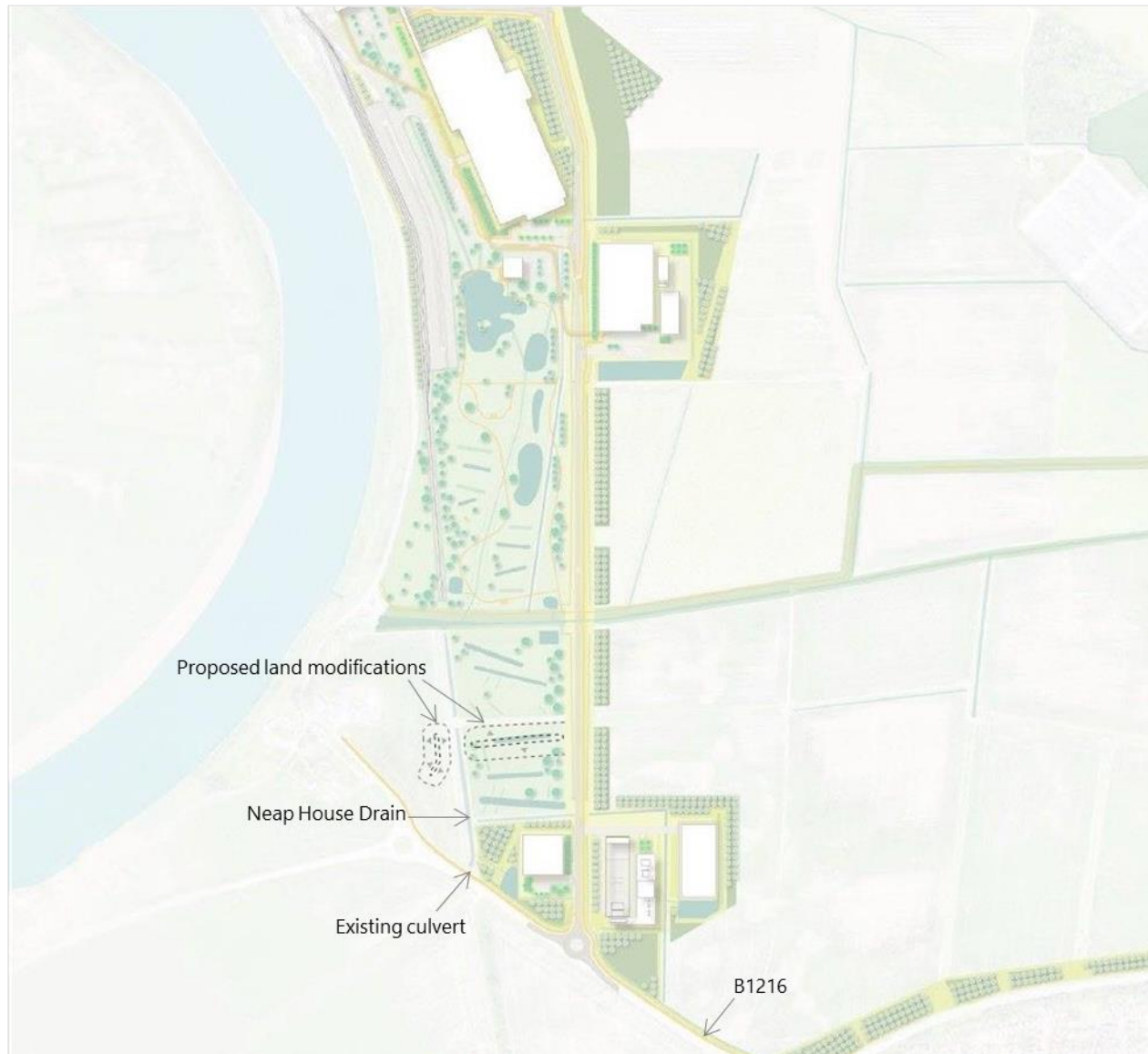
Figure 5.19 Plan view of location and footprint for proposed modifications to existing land levels (dashed lines indicate top and bottom of embankment).
