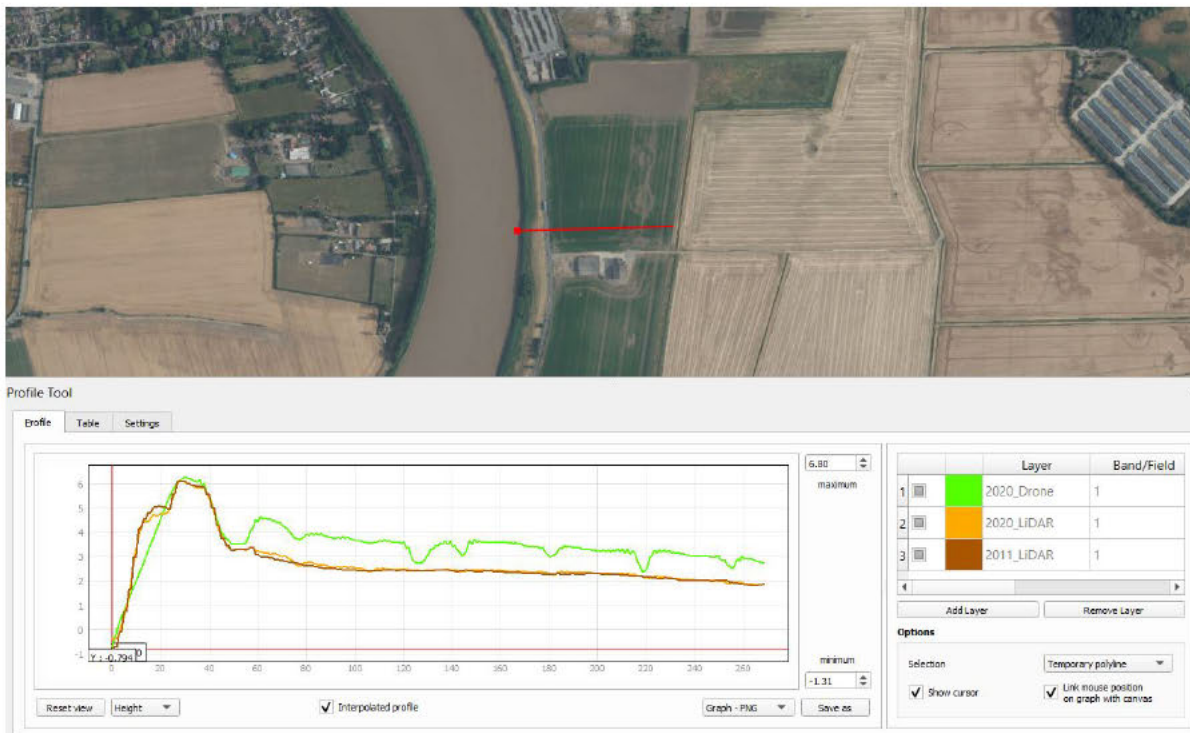
Figure 2.6 Profile sections along the east bank of the River Trent (top) and across the east bank (bottom) comparing the different datasets (Image courtesy of Ordnance Survey, © 2021 TomTom).
