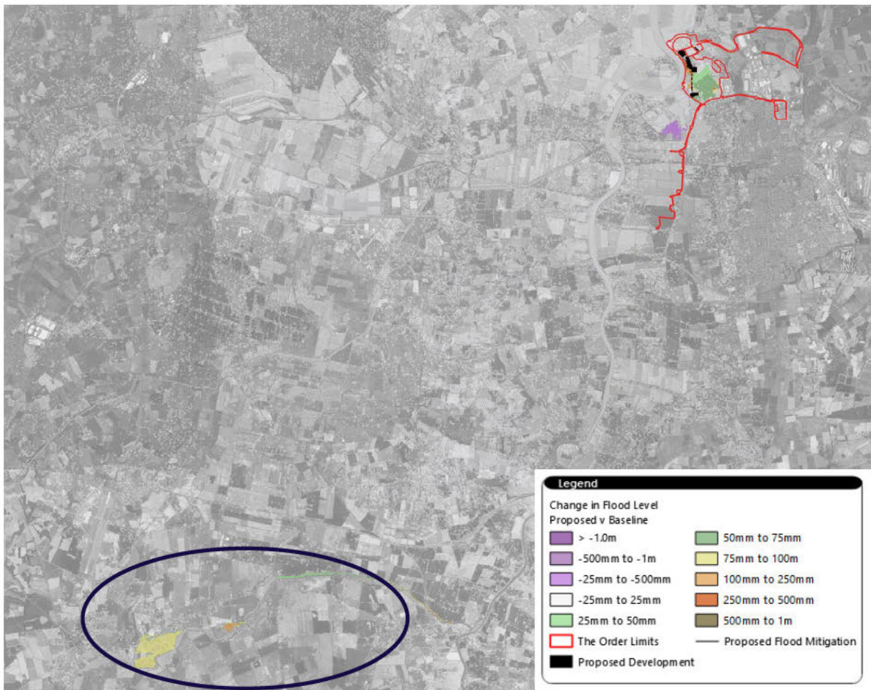
Figure 4.4 Image showing change in peak flood level due to proposals with mitigation Breach 02 versus baseline Breach 02 model. Change greater than 30mm to 100mm outside of the Project circled in blue (Image courtesy of Ordnance Survey, © 2021 TomTom).
