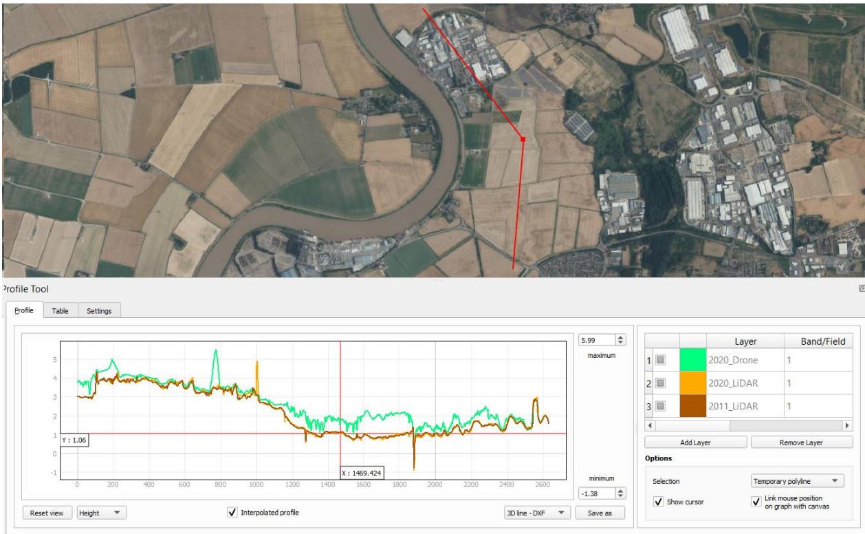
Figure 2.2 Long section profile through the Site comparing the drone survey flown 2020. LiDAR flown in 2020 and the Lidar flown in 2011 used in the NLC 2017 model (Image courtesy of Ordnance Survey, © 2021 TomTom).
